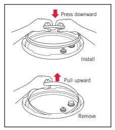
Figure 1. Removing and reaffixing the sealing gasket.
